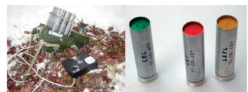
Initiating of shells Power supply autonomous from its own battery or lighter car Battery type - BB BATTERY BP7-12 (12V, 7AH/20HR) Voltage time to initiation LET & LEC after launch time to initiation LEFL after launch
